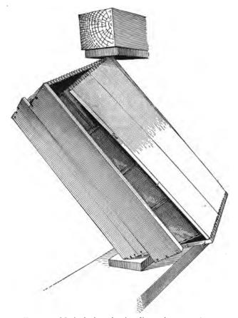
Fig. 47.—Method of conducting diagonal compression test.
